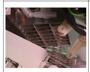
A thermistor temperature of -9.4°F signals the control board to begin harvest and energize the hot gas valve and actuator motor circuit. The actuator motor now turns counter clock wise to lower the water pan. The switch lever moves the actuator toggle switch to the left. This sets the actuator motor circuit to raise the water plate at the end of harvest. The board energizes the inlet water valve.
